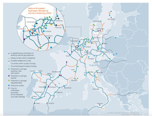
The map illustrates the vision for the hydrogen network in Europe according to the Hydrogen infrastructure – the pillar of energy transition publication.
