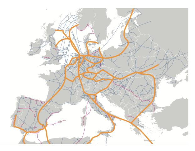
The map above shows the European Transnational Hydrogen Backbone - The natural gas infrastructure in Europe (blue and red lines) and an outline for a hydrogen backbone infrastructure (orange lines). The main part of the hydrogen backbone infrastructure consists of re-used natural gas transport pipelines with new compressors.
