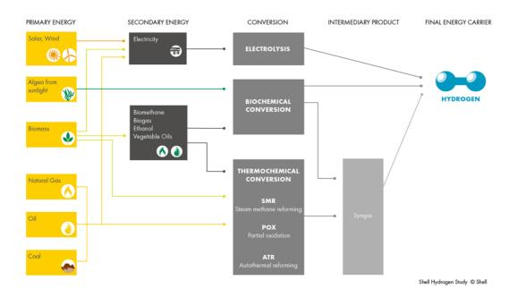
The figure above, from Hydrogen Europe, illustrates methods on creating hydrogen
